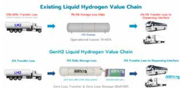
Figure 3. The existing liquid hydrogen value chain as compared to zero-loss, controlled storage Tank and an IRAS System.
